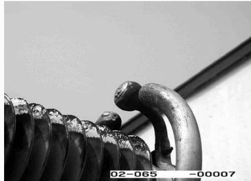
Figure 12.2: End Fitting after Power Arc Test
