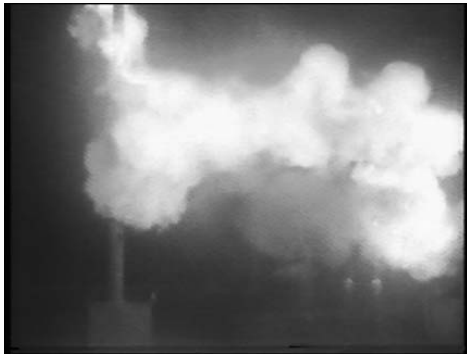
Figure 12.1: Arc Extension during Test
