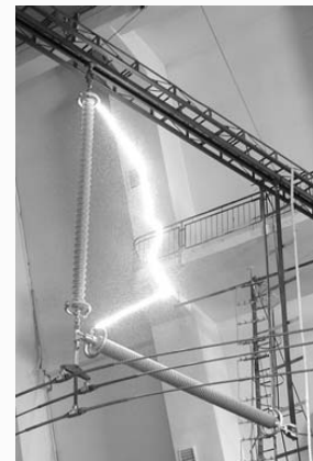
Figure 10: Wet Switching Impulse Testing
