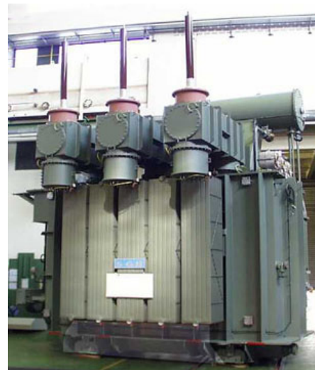
Figure 8: High-Voltage test and jumper terminal on the high voltage side of a power transformer (transformer SGB Regensburg).
