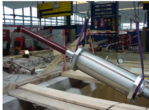
Figure 11: Test joint box with plug-in test adapter.
