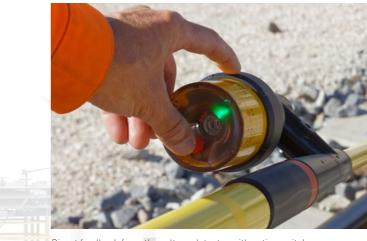
Direct feedback from the voltage detector with active switch-or
