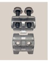
**Figure 1: Ideal arrangement of the contact elements:** Donati's rule of current commutation shows that the current density of a connection is not the same at all points: The commutation takes place for the most part at the beginning and at the end of the overlapping surfaces of the conductors. Ergo: The contact areas (zones, lines, points) are placed as close as possible to the beginning or end of the clamp.
