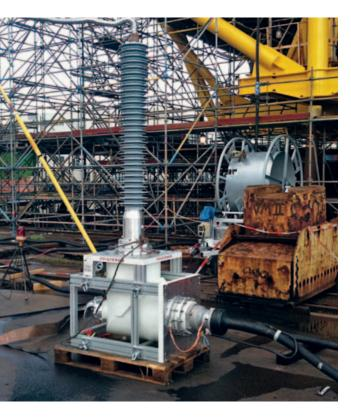
A key component: The transition from the overhead line to the test cable – using a modular assembly made up of elements of the HV-CONNEX system.
