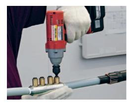
Only certain impact wrenches are suitable for the installation of shear off bolts.
