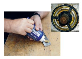
Contact protection paste prevents the oxidation of the points of contact.
