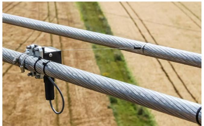
PT1 sensor for sub span oscillation measurement
