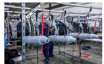
PFISTERER has developed a turnkey GIS bypass solution for rapid deployment in the Canary Islands and Balearics. It enables REE to secure the energy infrastructure on the isolated islands against system failures. 54 cable drums with pluggable HV connections are ready for immediate use in 18 shipping containers.
