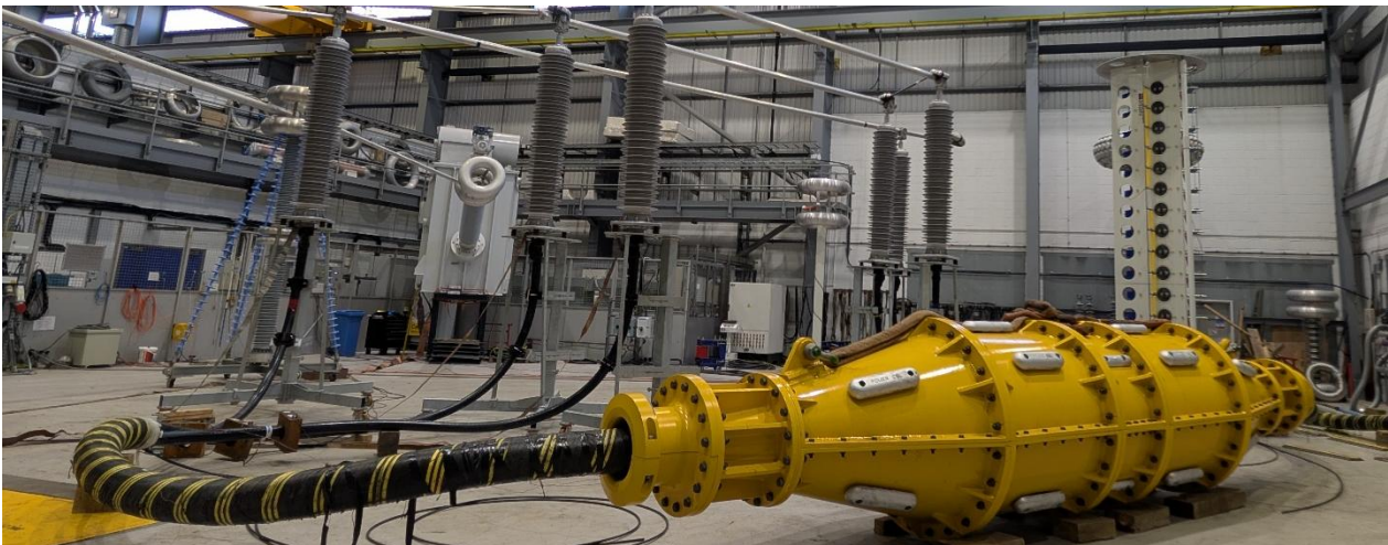
The universal repair joint allows the connection of a wide variety of HVAC subsea cable types using the plug-in principle – completely independent of the design or manufacturer of the cables used. Source: PFISTERER
